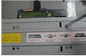
5. Use screws to fix HDD.
