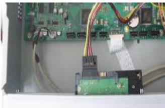
8. Insert the HDD power cable.
