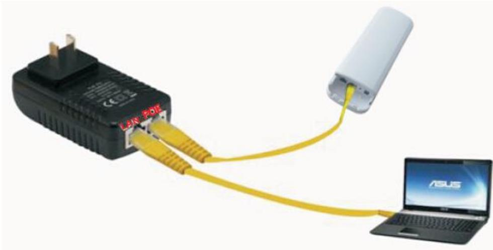
P2 Connection diagram of CPE and PoE adapter
