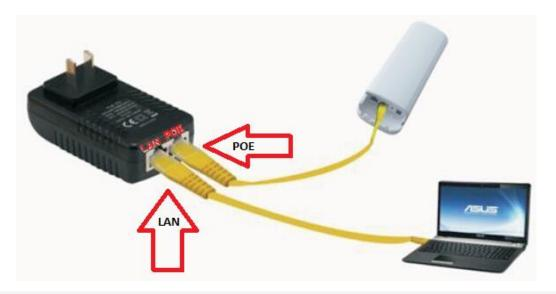
P2 Connection diagram of CPE and PoE adapter
