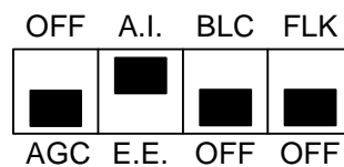
Figure 5. Switch for camera mode (HW V1.5 or later version)
