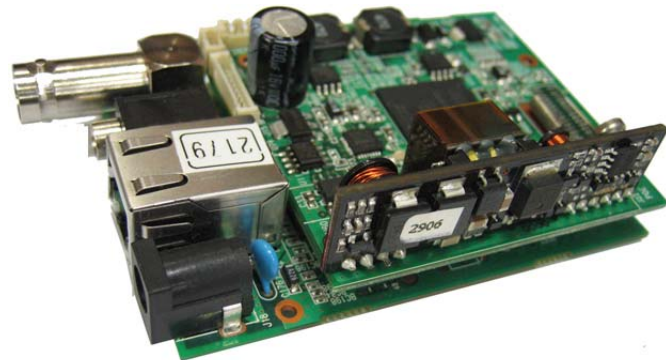
Figure 19. IPC1100 with PoE module installed
