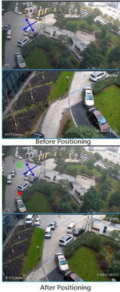
Figure 3-172 3D positioning (Zoom out after positioning)
