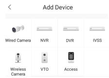
5. To add a device using IP address of the device itself, follow step# 2 but this time select IP/Domain then select correct device type as mentioned above at step# 4.
