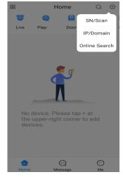
3. Scan the Device SN QR code from the recorder as mentioned on step# 1. To manually enter serial number, tap "Manual Enter SN".
