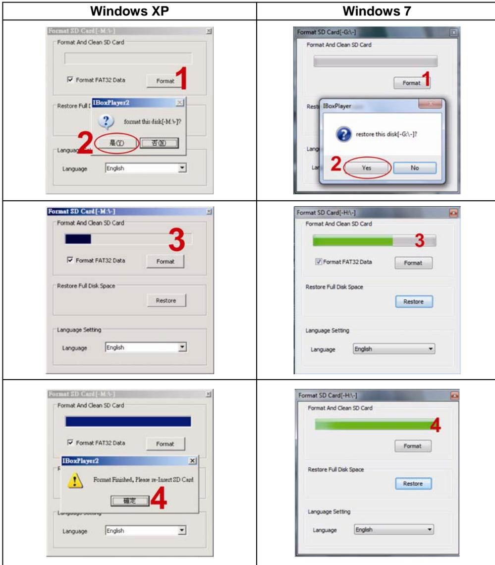
3. When formatting is completed, please insert the card into the machine for recording.
