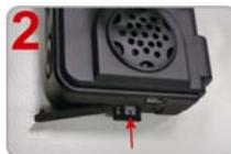
Insert the Micro SD card in correct direction.
