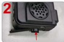
2 Insert the SDHC card in correct direction.
